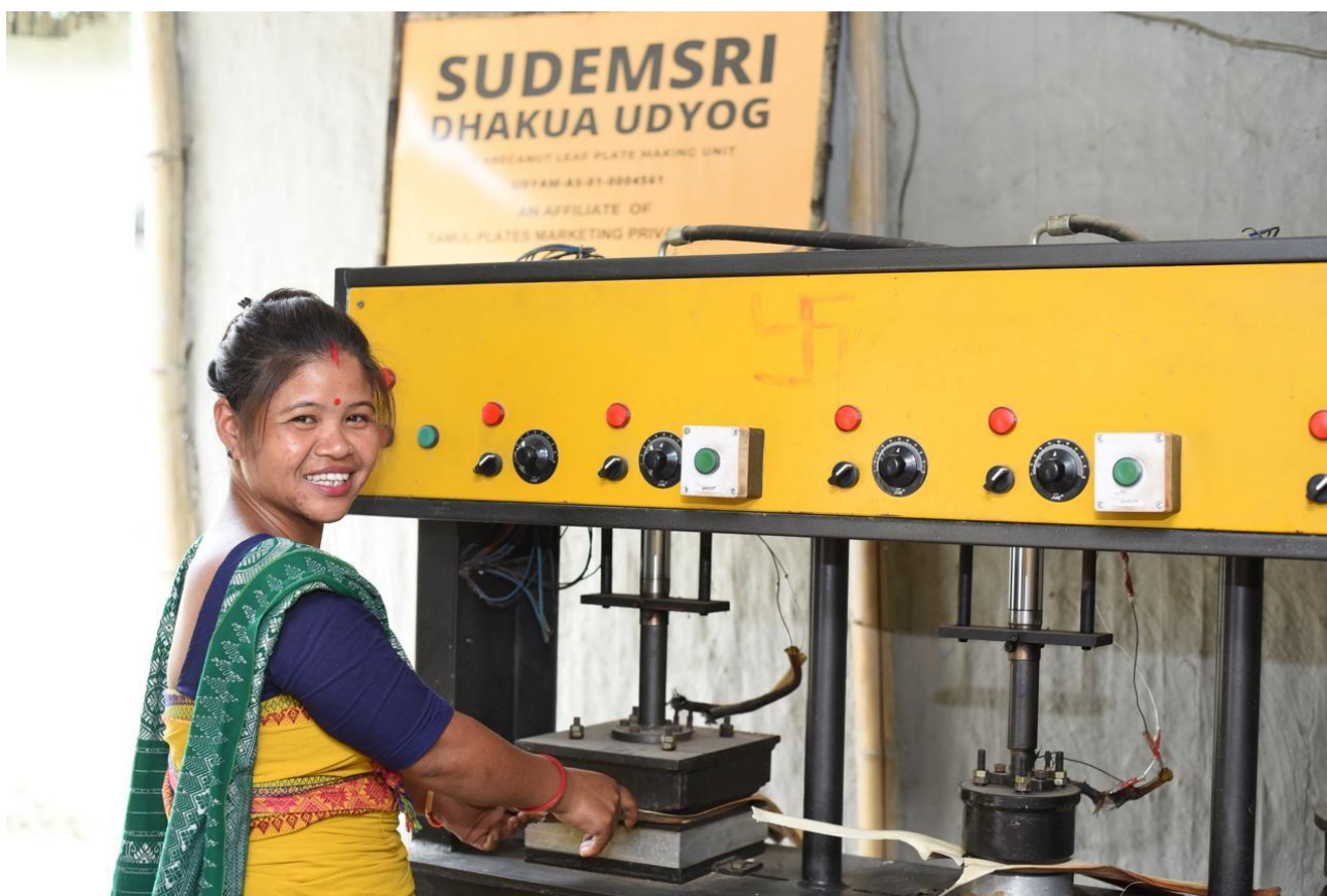
Figure 11 A member of the Sudemsri Dhakua Udyog (a 5 member JLG) operating her arecanut leaf plate making machine in her time slot
